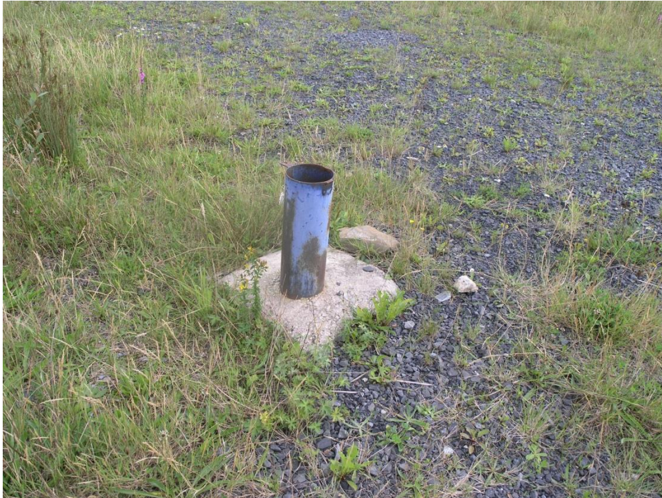
Figure 13.14: Groundwater monitoring well in situ
